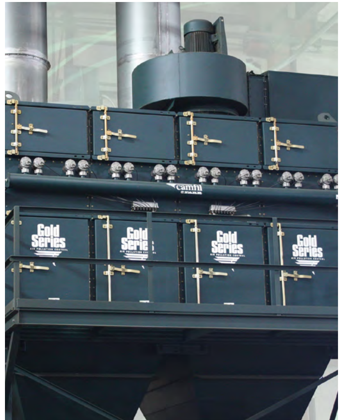
HEPA safety monitoring filters are integrated on top of this dust collector, eliminating the costs of additional ductwork. Mounted downstream of the HEPA filters, the fan is protected against wear and tear from exposure to abrasive silica particles.
