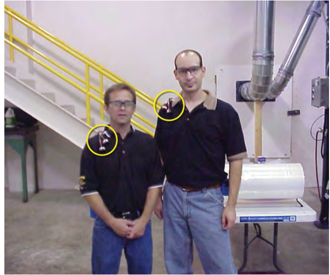
OSHA accepts several methods of air monitoring to determine worker exposure to silica dust – including personal air sampling as shown in photo.
