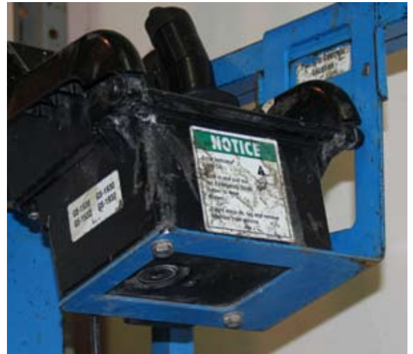
Damaged or deteriorated labels, like the one above, need to be replaced.
