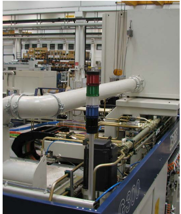
This machining center is equipped with high efficiency collection equipment designed for removal of emulsion coolant mist.
